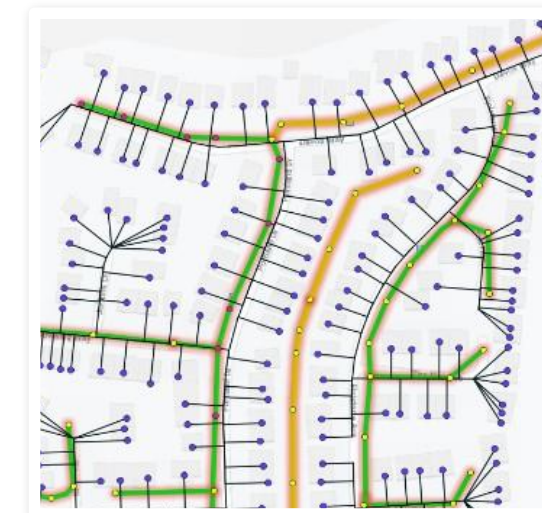
Figure 3: Sample of pathfinding simulation with correlated cost based on existing infrastructure
