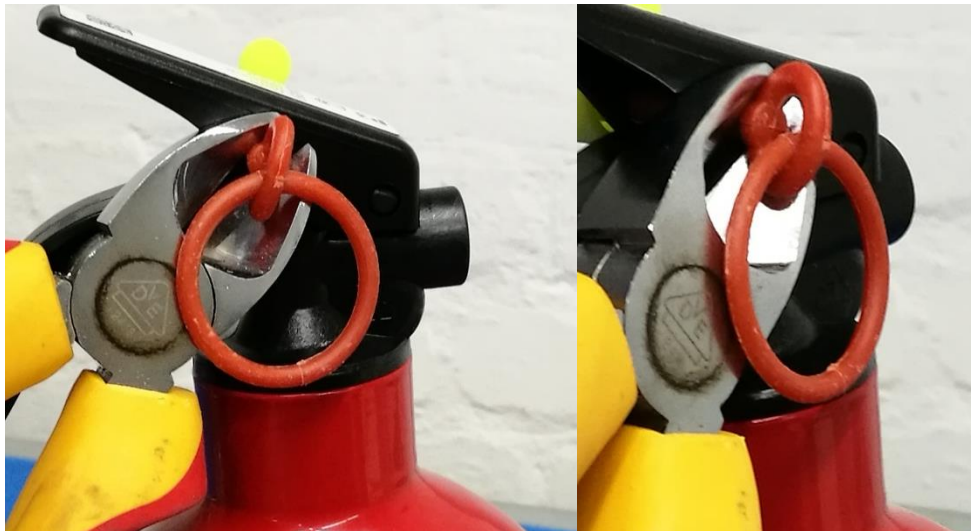
Figure 1: Cutting the safety pin (left)
