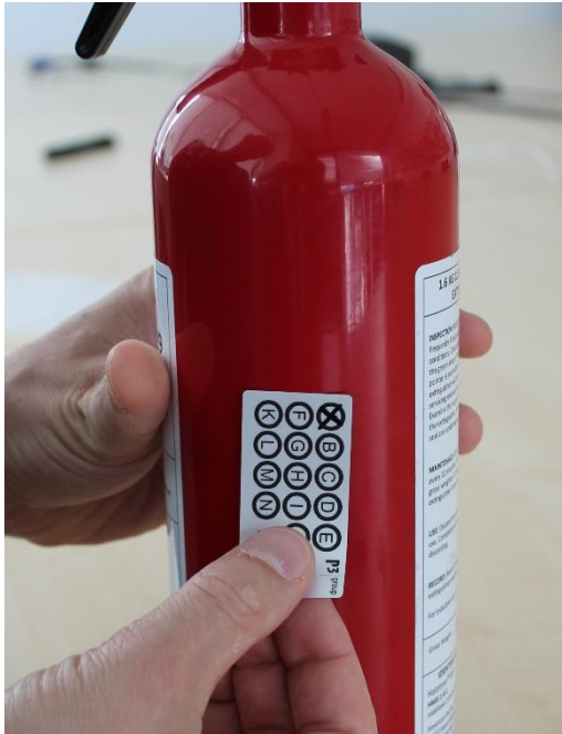
Figure 4: Placing the amendment plate
