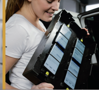
Each drive test vehicle carried nine smartphones for the voice and data tests.
