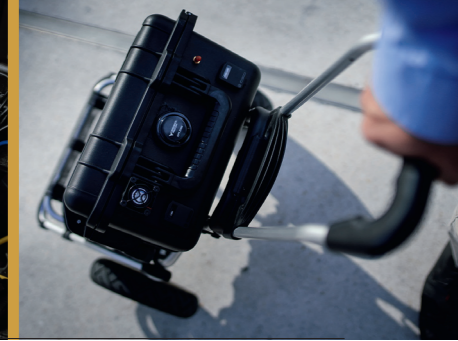
The walk test teams used trolleys or backpacks with powerful batteries to power the test smartphones.
