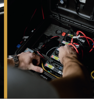
A special control system monitors the test smartphones and logs the measured values they record.
