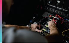
Each drive test car carried nine smartphones for voice and data testing. The walk test teams had trolleys equipped with powerful batteries to power the test smartphones.
