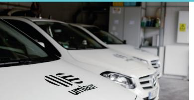
The measurements in Germany took place from 14 to 27 October 2025, in Austria from 9 to 27 October 2025 and in Switzerland from 13 October to 1 November 2025. For each country, connect network test partner umlaut sent four measurement vehicles onto the road, each equipped with nine smartphones.
